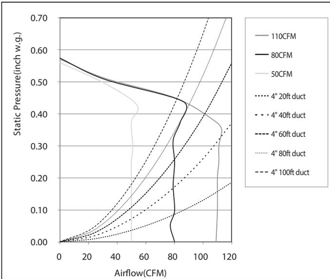
**Performance Curve** FV-0511VFC1 - 3" Duct
