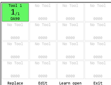
The unit will return to the Tools screen with the just learned tool now with a tool name of “Tool 1” instead of “No Tool”.
