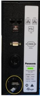
Plug the provided power cable into the unit and 100-240 VAC power and turn on the power switch. The beeper will sound a series of quick beeps and the display will show the loading progress.
