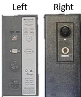
The left side of the EYFR04 has two RJ-45 Ethernet ports to allow it to be used in a chain network configuration.
