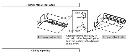
Install inspection opening 17 23/32" x 17 23/32" (450 mm x 450 mm) on the control box side where maintenance and inspection of the control box and drain pump are easy. Install another inspection opening 31 1/2" x 27 9/16" (800 mm x 700 mm) also at the lower part of the unit.
