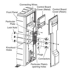
8 Connect the power supply cord and connecting wire between indoor unit and outdoor unit according to the diagram below.
