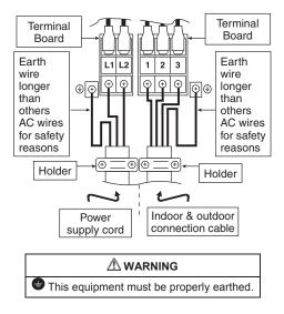
• Earth lead wire shall be Yellow/Green (Y/G) in colour and longer than other lead wires for electrical safety in case of the slipping.
