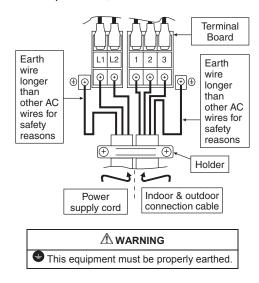
• Earth lead wire shall be Yellow/Green (Y/G) in colour and should be longer than other lead wires as shown in the figure for electrical safety in case of slipping.
