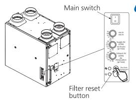
After re-connecting power, and turning on the main switch, press the filter reset button about 3 seconds to reset run timer.
