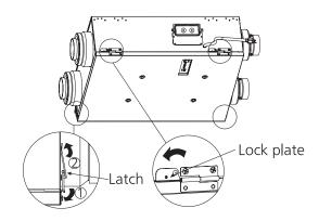
Reinstall and close frame cover by locking the latches, then reset the lock plate.
