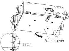
2 Open the frame cover by unlocking the latches.
