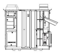
Remove Outside Air (white paper) filter and Return Air (black resin) filter to clean with vacuum cleaner.
