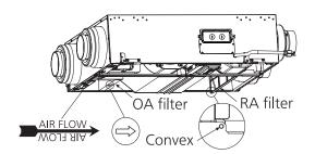
Replace the Outside Air (white paper) and Return Air (black resin) filters. Make sure the Return Air (black resin) filter adapts to the convex and the direction of the arrow on the Outside Air (white paper) filter is in the same direction as the air flow displayed on the nearby label.
