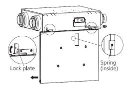
Remove Outside Air (white paper) filter and Return Air (black resin) filter to clean with vacuum cleaner.
