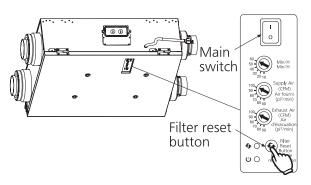
After re-connecting power, and turning on main switch, press the filter reset button about 3 seconds to reset run timer.
