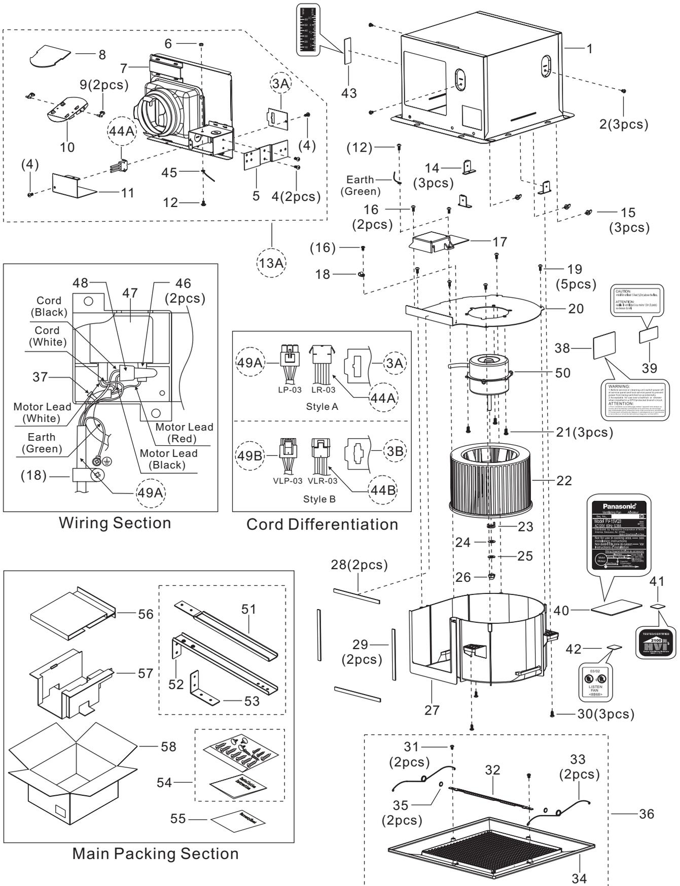
Remark: Please take attention to the parts which circled with broken line, We express the different style parts in using a letter marked behind a number, such as 3A means the item 3 belongs to style A.
