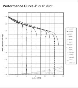
\*Industry research indicates static pressure in typical installations ranges from 0.20" to 0.375"
